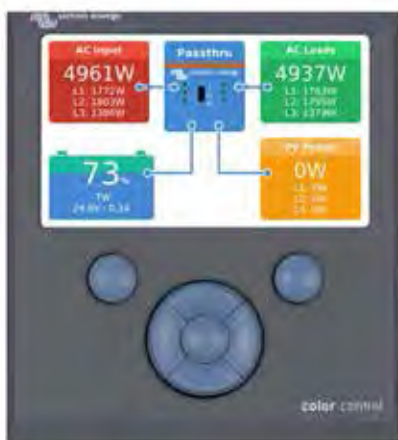
Color Control panel, showing a PV application
